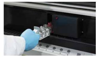
Onboard barcode reader allows real-time reagent management.
